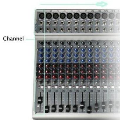
I start with channel 1 where the INPUT is my microphone. Moving down, I adjust my GAIN around 0 to -15. I do this because the gain controls the input level of each individual channel. Now I can push my channel fader all the way up to 0. Faders control the level of each channel sent to outputs, like master.
